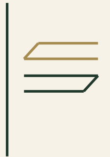
French cleat - side-view concept
